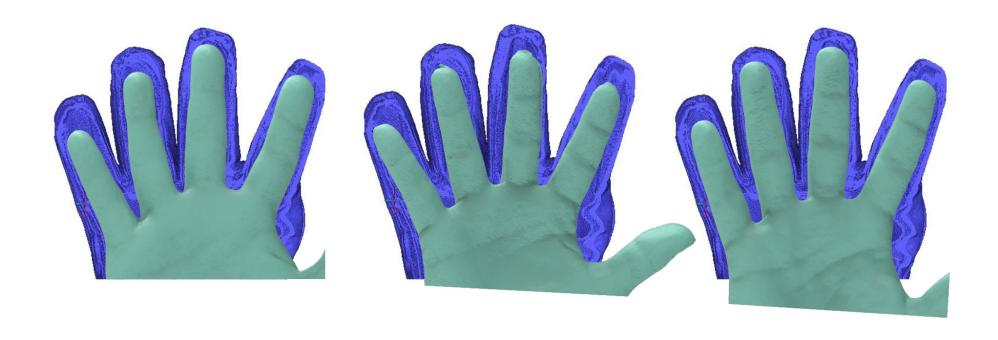
Image 3. Glove Interior-Hand Comparison; Using CT Scanning, glove interior can be captured with high dimensional accuracy. 3D hand scans are aligned with the cross-sections of CT scan data to understand the differences between glove webspace and hand crotch slope.
