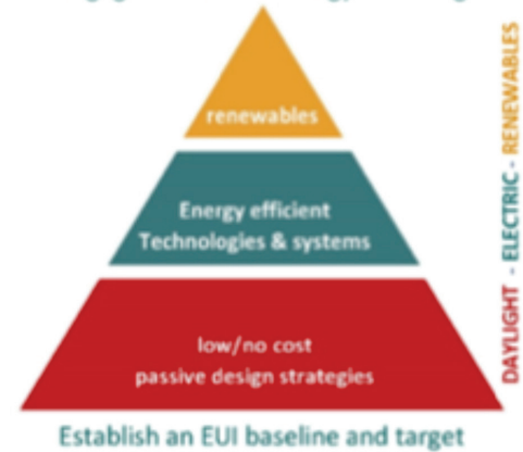
Figure 3: Net-Zero Energy Design Hierarchy (Credit: Author, based on "Zero by2040", Architecture 2030).
