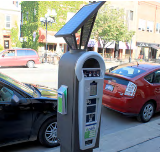
Figure 75: Solar-powered smart meter in Ann Arbor MI
